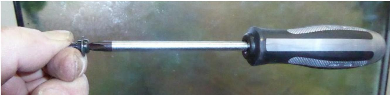
No trick. The screw is a Honda cross head screw with a small shoulder. The sort that you will find two of at the front of the fairing pocket, or fastening the fairing behind the mirror housing. The screwdriver is a Pt2 JIS Vessel driver, like the middle of the three shown above, except this one has an impact driver mechanism built into the handle. It has the same driver point as the normal one, but it has a much heavier handle. Bash the end with a hammer, it turns the screw a fraction.
