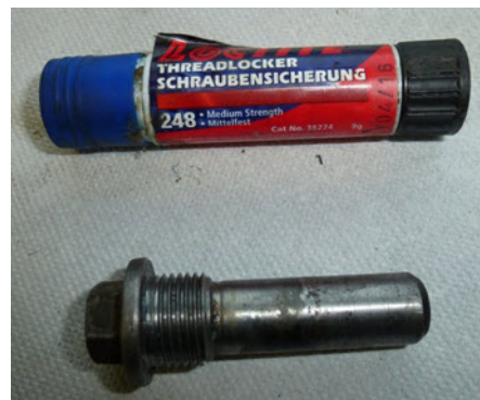
Blue thread locking compound from Halfords. Don't use the red stuff (UK) - it locks the thread completely.
