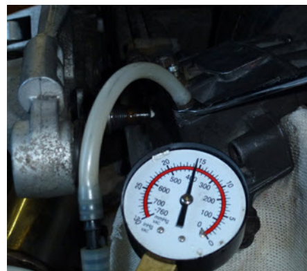
A vacuum pump attached to the rear bleed nipple of the rear caliper
