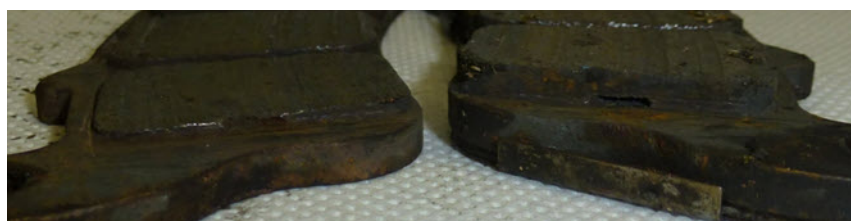
A pair of rear brake pads. The left side has worn to the limit notch - just visible on the friction pads. The right still has some wear left. Something is wrong here, the amount of wear should be roughly the same.
