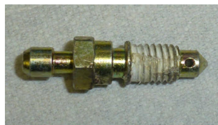
A new bleed nipple with PTFE tape wrapped round the thread. Worth doing if you intend to use a vacuum pump.
