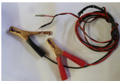
Home made Inspection Harness
