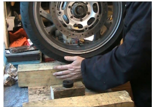
Step 2 - Have supports to lift the disk away from the surface, and a central 'anvil' for on which the removal tool will rest while the drift is located.
