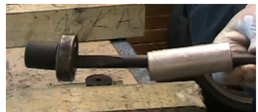
Step 4 - The removed bearing with removal tool and drift still wedged inside. Don't loose the spacer !
