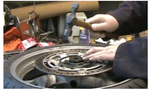
Step 1 - Right hand side first. Tapping the bearing home using a solid metal disc. The correct handle and pilot had not arrived in time for this photo !
