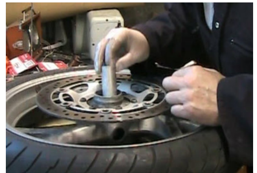
Step 2 - Turn the wheel over and insert the spacer. Make sure it sits on the face of the bearing just installed.
