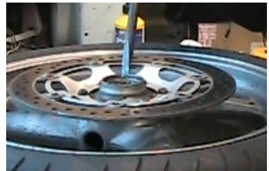
Step 3 - Locate the drift, remove the anvil and start tapping it out.
