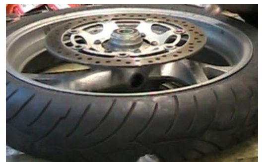
Step 3 - Bearing waiting to be driven in. Use the proper tool, or beware driving the bearing beyond the top of the spacer. Or not enough.
